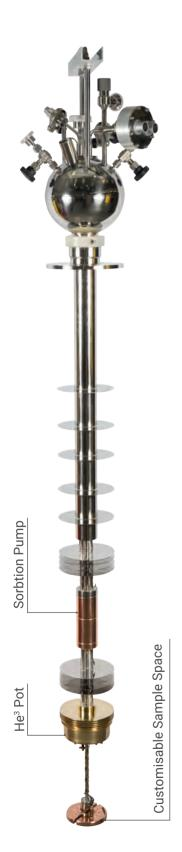
The ICE <sup>CP</sup> 300mK Cold Probe is a compact, fast turnaround insert available for top loading systems into a Variable Temperature Insert (VTI) or for continuous flow systems.
