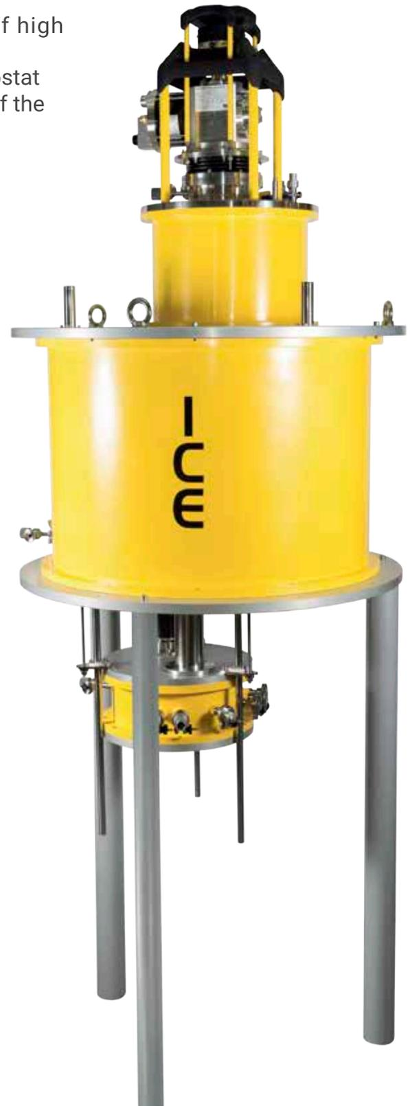
Total height requirement for system operation: 1550mm
